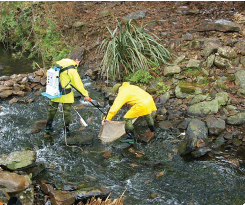
NIWA representatives demonstrating electric fishing to Kaitiaki one of the methods used to monitor and survey tuna. (Photo and caption provided by Te Rūnanga o Te Rarawa)
